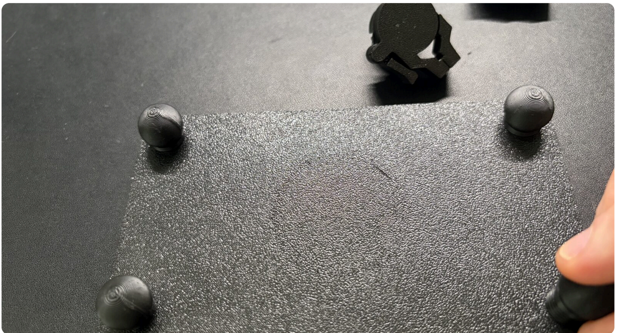
Ball joints screwed into the top face of the jig
