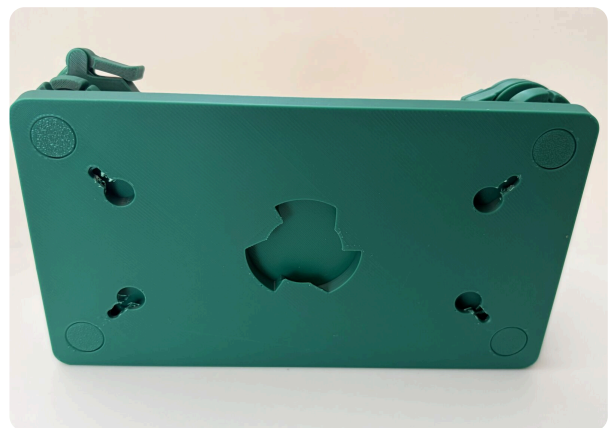
Keyhole hangers on the underside of the jig
